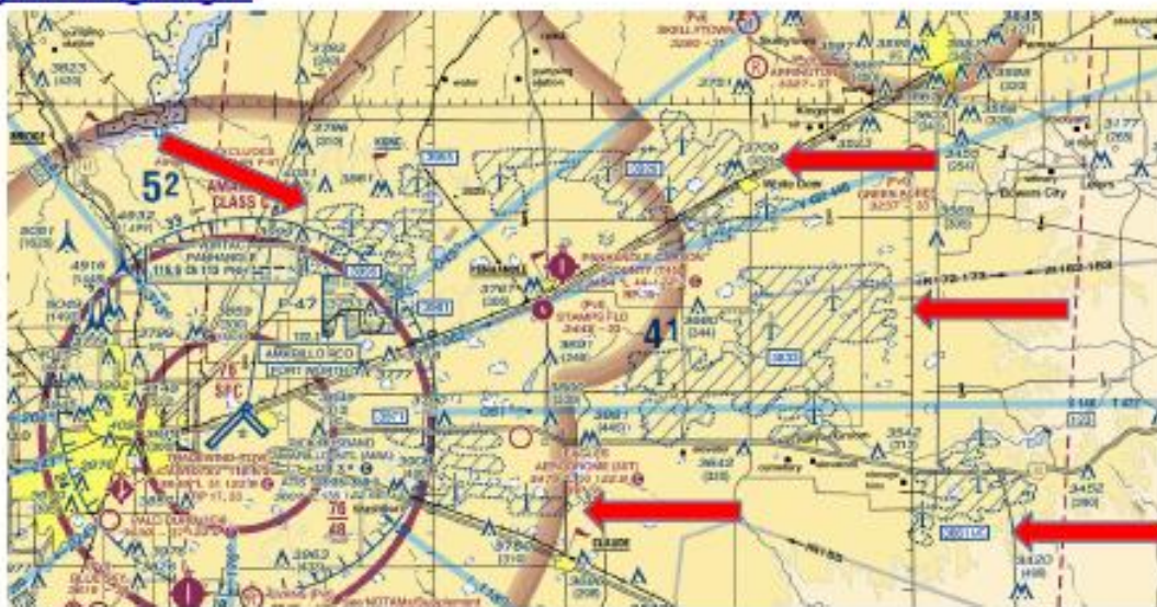
A few examples of Wind Turbine Farms with enhanced depiction near Amarillo, TX (Dallas-Ft. Worth VFR Sectional Chart.)
